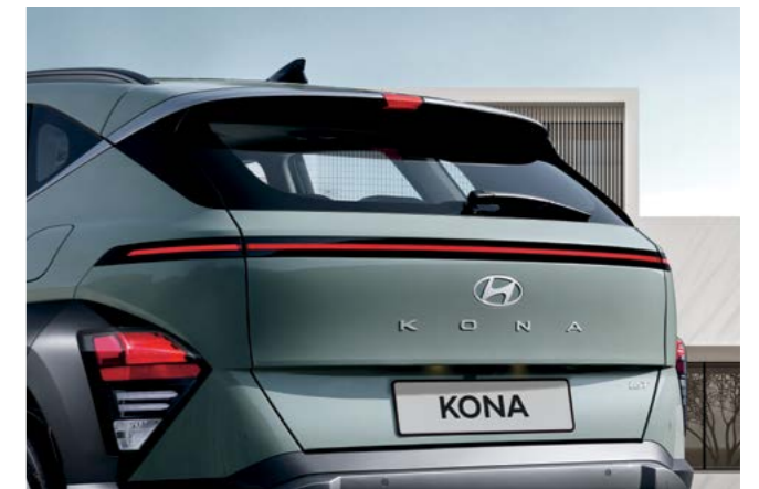
Spoiler integrated HMSL, rear seamless horizon lamp LED brake lamps, LED turn signal lamps
