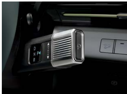
Electronic Shift-By-Wire (E-SBW) column type gear selector
