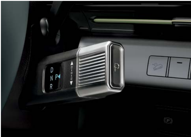
Column-Type Electronic Shift by Wire (E-SBW)
